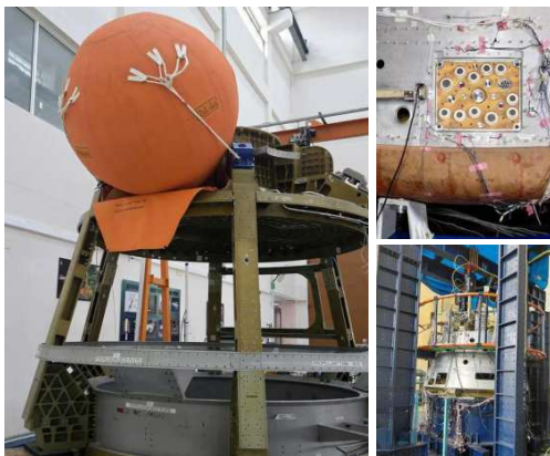
Step-by-step: (Clockwise from left) The crew module uprighthing system, the service module connect-disconnect system, and the apex cover that underwent testing. ISRO
